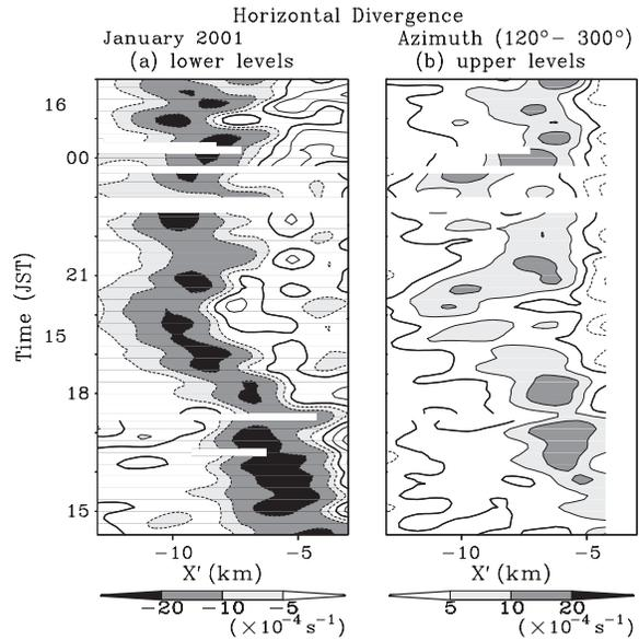
Fig. 13. Time-distance cross sections of the horizontal divergence in  $10^{-4} \text{ s}^{-1}$  derived from RHI scans of an orientation of  $120^\circ$  and  $300^\circ$ . (a) Lower levels (averaged for the height between 0.25 km and 0.75 km). (b) Upper levels (averaged for the height between 1.5 km and 2.0 km). The right-hand side of the figure is the landward side. The contours are drawn at  $-20, -10, -5, 0, 5, 10,$  and  $20 \times 10^{-4} \text{ s}^{-1}$ .
