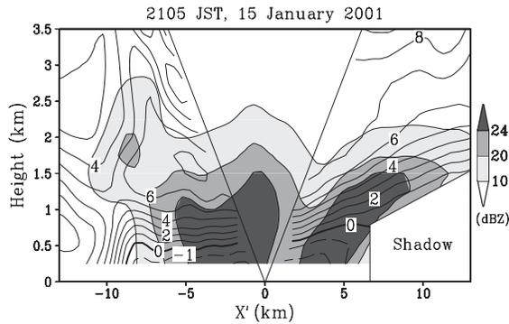
Fig. 14. Vertical cross section of the reflectivity (gray levels, dBZ) and horizontal wind (contour lines,  $\text{m s}^{-1}$ ) in the cross section derived from the RHI scan with an orientation of  $120^\circ$  and  $300^\circ$  at 2105 JST, 15 January 2001. The right-hand side of the figure is the landward side. The positive velocity indicates the wind blowing from the sea to the land.
