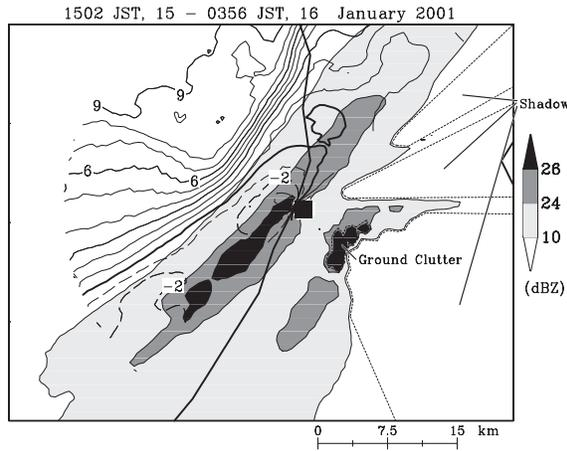
Fig. 12. CAPPI display of the time-averaged Doppler velocity (contour lines,  $\text{m s}^{-1}$ ) at a height of 0.25 km and time-averaged reflectivity (gray levels, dBZ) at a height of 0.5 km from 1502 JST, 15 to 0356 JST, 16 January 2001. The contours are drawn every  $1 \text{ m s}^{-1}$ . The positive Doppler velocity represents the wind approaching the Oshimizu radar marked with  $\blacksquare$ .
